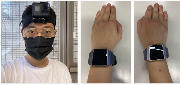
Fig. 2. The devices used to collect the data. A GoPro 5 camera is mounted at the subject’s head and two Fitbit Ionic watches are installed on two wrists.
